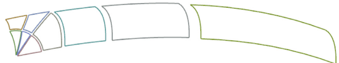
Fig. 51. Subdivision of curved slender quadrilateral element with BTSM with source point at (-1.0, -1.0).
