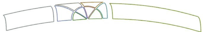
Fig. 52. Subdivision of curved slender quadrilateral element with BTSM with source point at (-0.2, -1.0).
