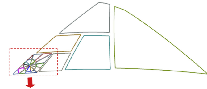
Fig. 45. Subdivision of curved slender quadrilateral element with BTSM with source point at (0.55, 0.85).
